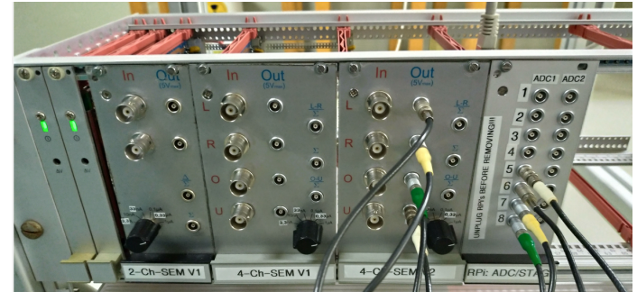
Calibration of SEM signal to proton beam current @ 1000.0 nA
