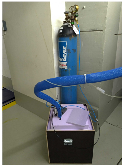
Liquid N 2 -reservoir for gas cooling and respective gas cylinder
