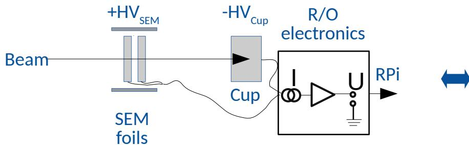
*Beam current calibration schematic setup*
