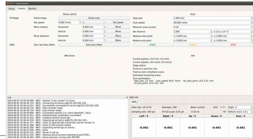
Interface for setting irradiation parameters and XY-stage control
