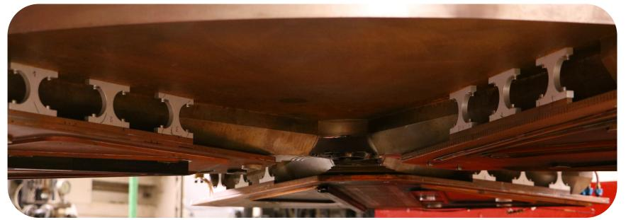
Magnetic yoke of the cyclotron
