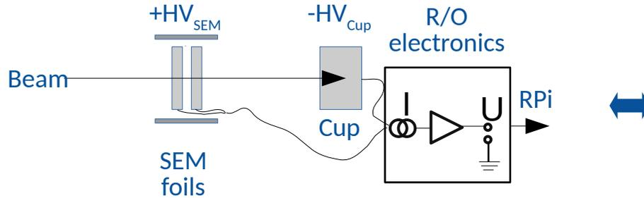
*Beam current calibration schematic setup*
