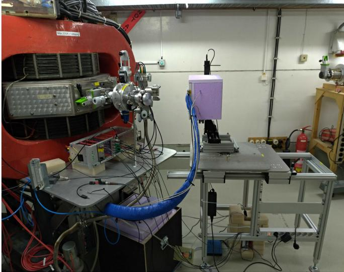
**Cooling:** irradiation in **cooling box**, N<sub>2</sub> gas cooling (in liquid N<sub>2</sub> reservoir) to prevent **annealing** effects. Temperature monitoring via NTCs at 2 positions.
